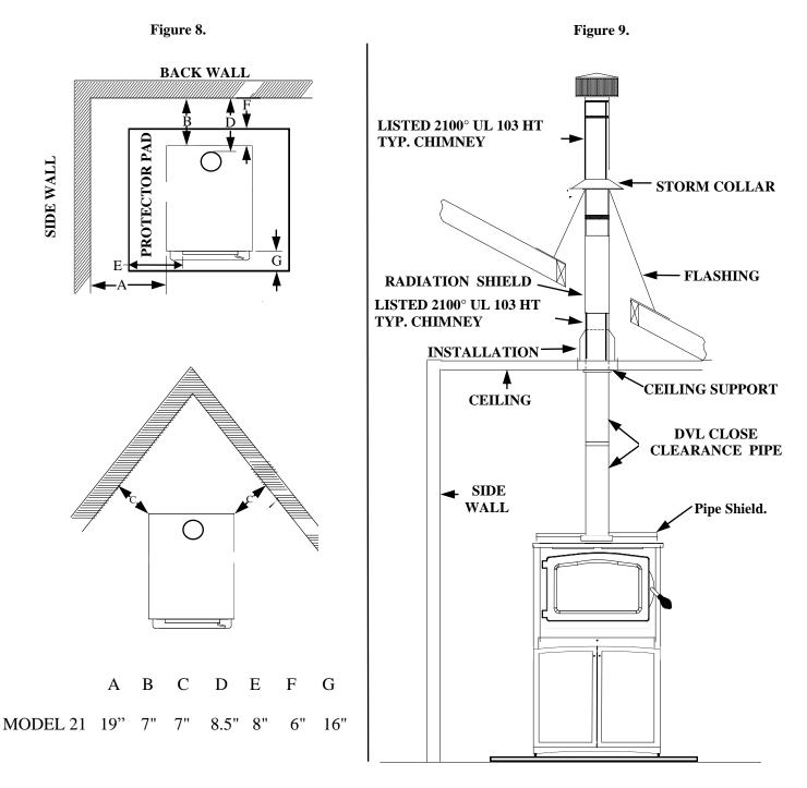
**NOTE:** All clearances are to combustibles with optional close clearance shields and pipe shield, using DVL Close Clearance pipe, and minimum floor protector.
