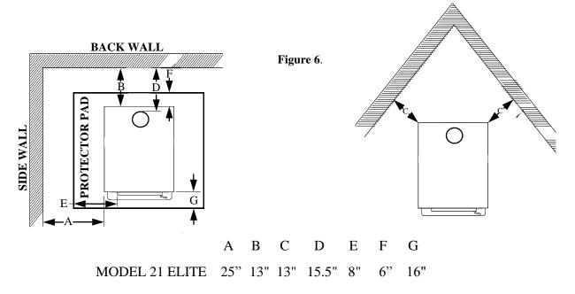
**NOTE:** All clearances are to combustibles with pipe shield, 6" Single Wall minimum 24 ga. blued or black pipe with elbow and minimum floor protector. Clearances above may be reduced. Follow **NFPA-211** codes if available or follow instructions on (Pages 13, and 14).
