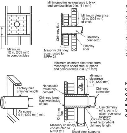
A) Minimum 3.5-in thick brick masonry all framed into combustible wall with a minimum of 12-in brick separation from clay liner to combustibles. The fireclay liner shall run from outer surface of brick wall to, but not beyond, the inner surface of chimney flue liner and shall be firmly cemented in place.
