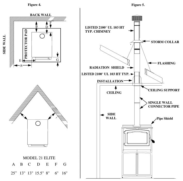
**NOTE:** All clearances are to combustibles without pipe shield, using 6" single wall minimum 24 ga. blued or black pipe and minimum floor protector. The clearances above may be reduced. Follow **NFPA-211** codes if available or follow instructions on (Pages 11, and 12).
