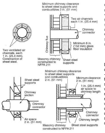
C) Sheet steel chimney connector, minimum 24 gauge in thickness, with a ventilated thimble, minimum 24 gauge in thickness, having two 1-in. air channels, separated from combustibles. by a minimum of 6-in. of fiber insulation. Opening shall be covered, and thimble supported with a sheet steel support, minimum 24 gauge in thickness.
