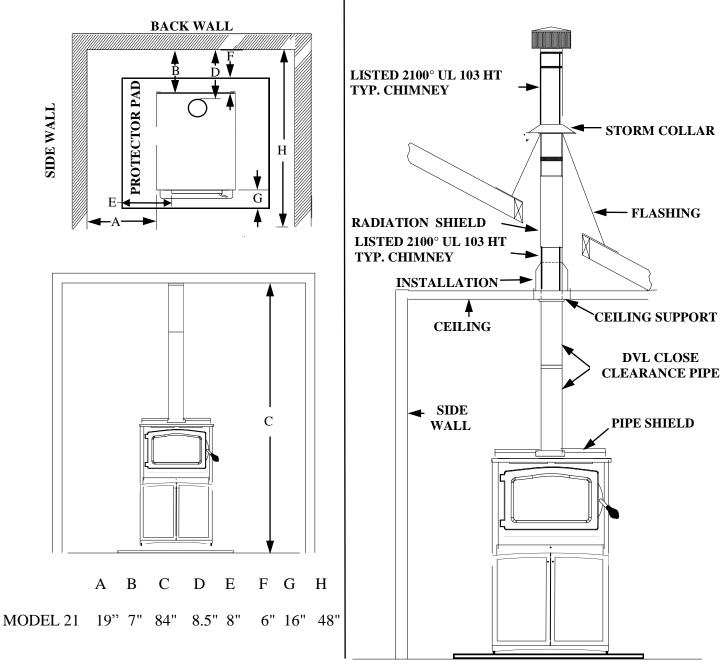
**NOTE:** All clearances are to combustibles with pipe shield, using DVL Close Clearance pipe and minimum floor protector.
