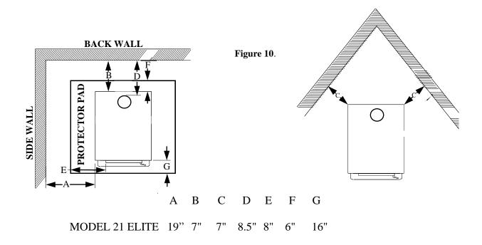
**NOTE:** All clearances are to combustibles with close clearance shields and pipe shield, DVL Close Clearance pipe with elbow and minimum floor protector.
